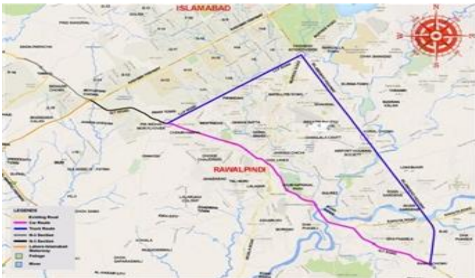
Figure 2: Alignment # 1 for the proposed Rawalpindi Bypass (60 Km)
